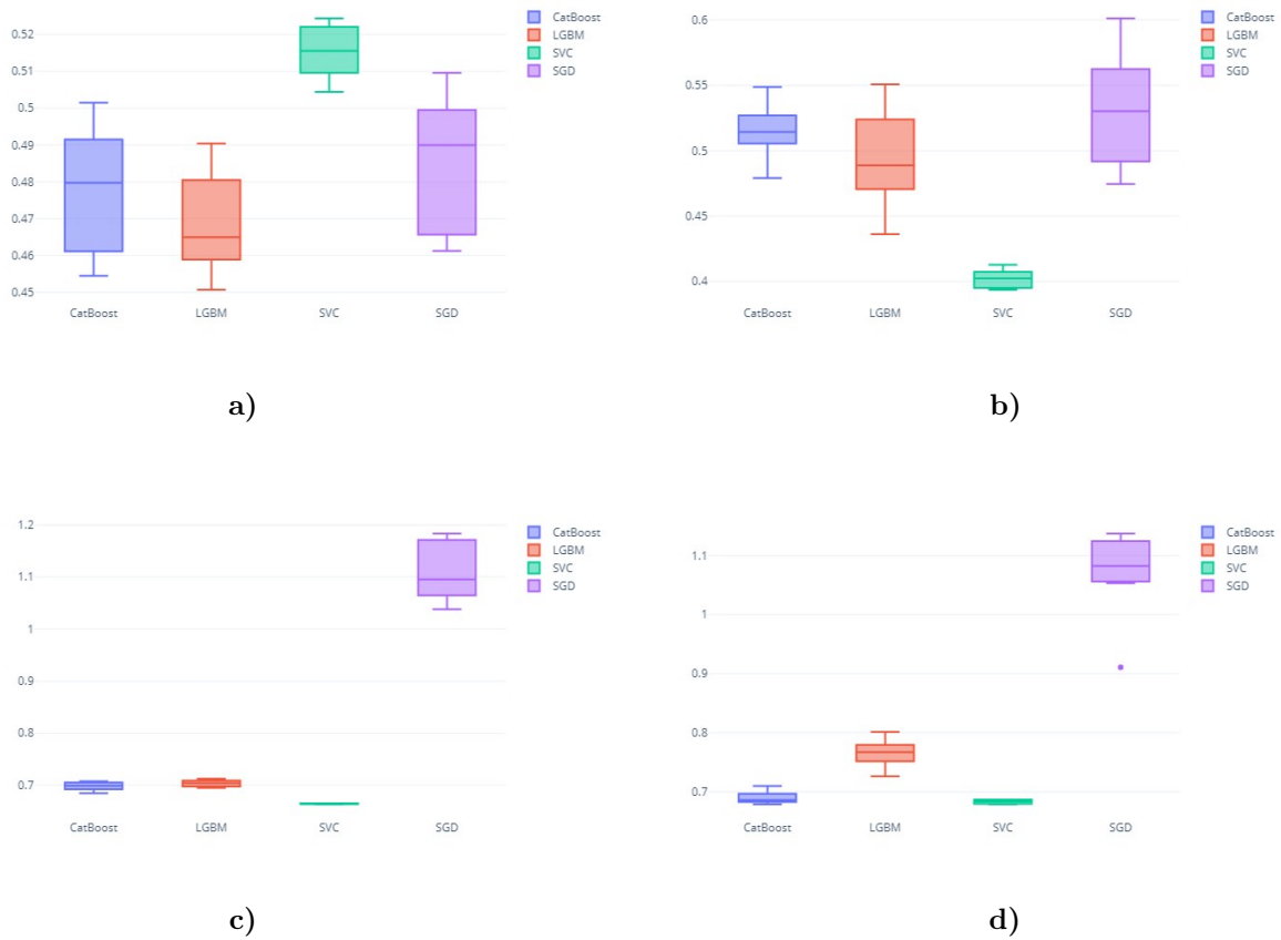
Figure 4.44: General overview of ROC-AUC (a and b) and Brier scorer (c and d) performance for the different predictive models. a and c refer to the cross-validation results, while b and d refer to the holdout results.
